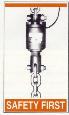
Automatic reset by reducing the load.
